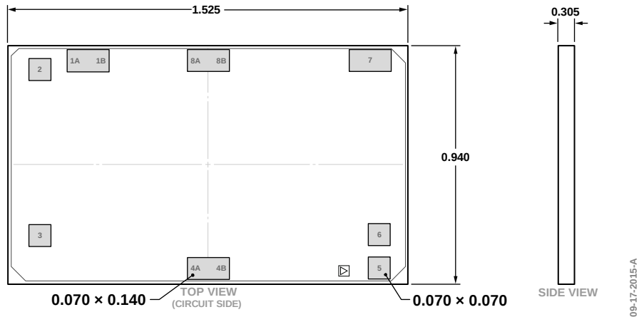
Figure 4. 8-Pad Bare Die [CHIP] (C-8-4) Dimensions shown in millimeters
