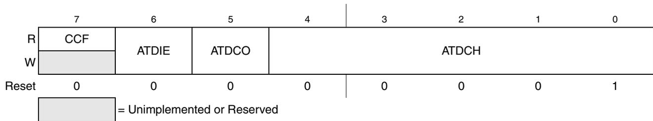
**Figure 14-6. ATD Status and Control Register (ATD1SC)**
