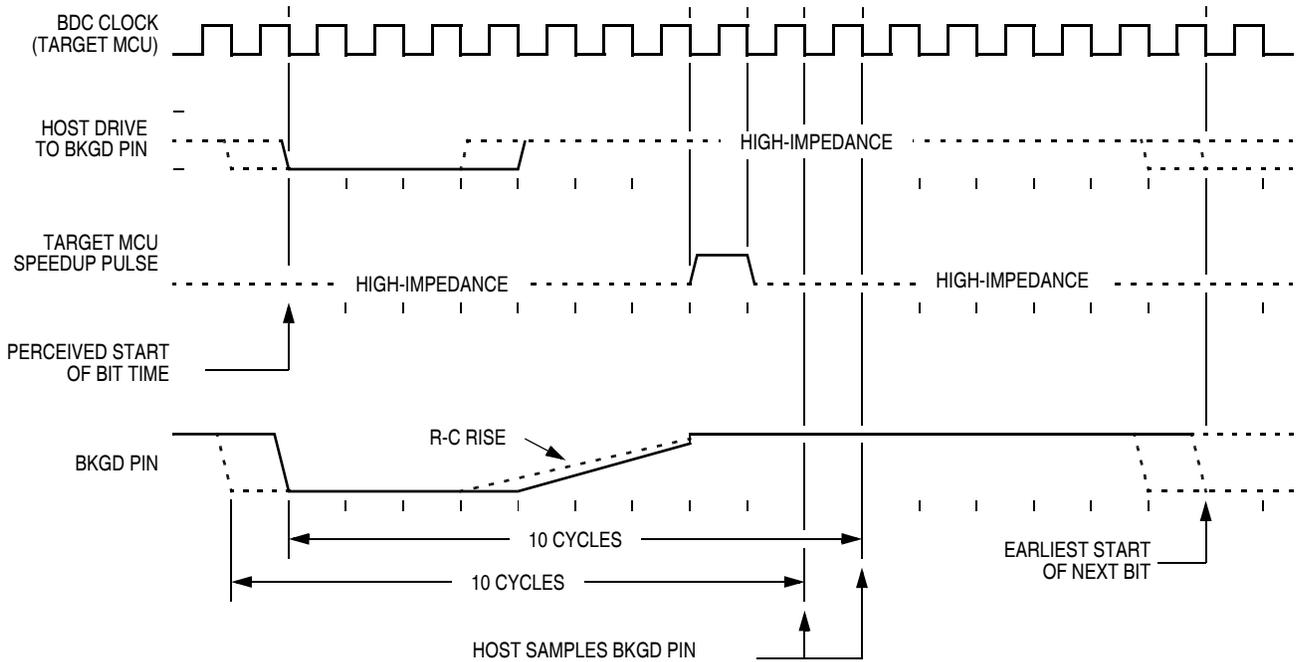
**Figure 15-3. BDC Target-to-Host Serial Bit Timing (Logic 1)**
