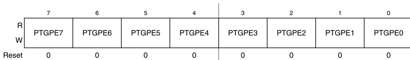
Figure 6-34. Pullup Enable for Port G (PTGPE)
