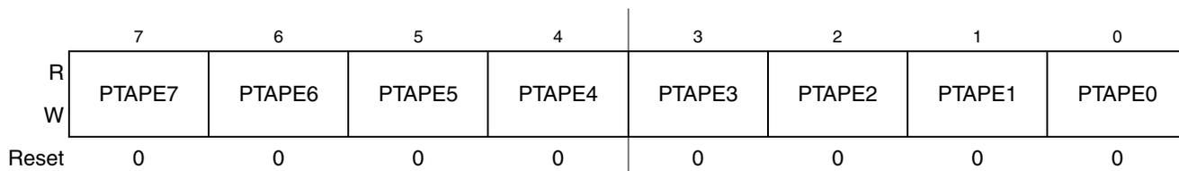
**Figure 6-10. Pullup Enable for Port A (PTAPE)**
