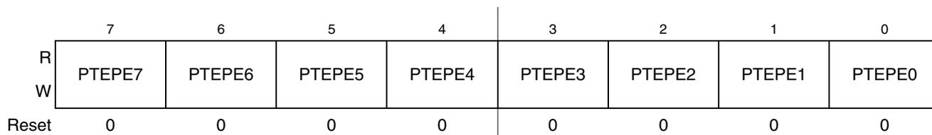
**Figure 6-26. Pullup Enable for Port E (PTEPE)**
