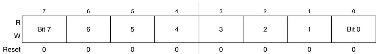
Figure 10-9. Timer x Counter Modulo Register Low (TPMxMODL)
