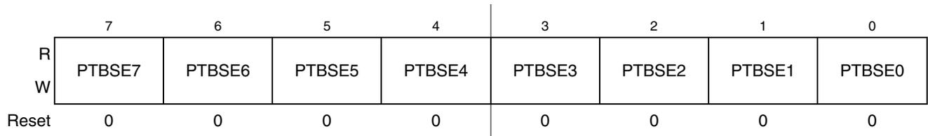
Figure 6-15. Data Direction for Port A (PTBSE)
