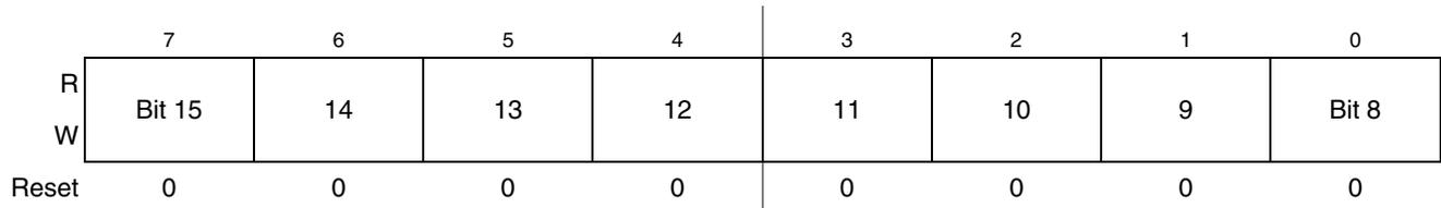
Figure 10-8. Timer x Counter Modulo Register High (TPMxMODH)
