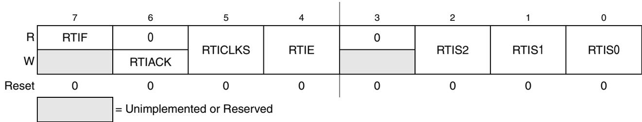
**Figure 5-8. System RTI Status and Control Register (SRTISC)**
