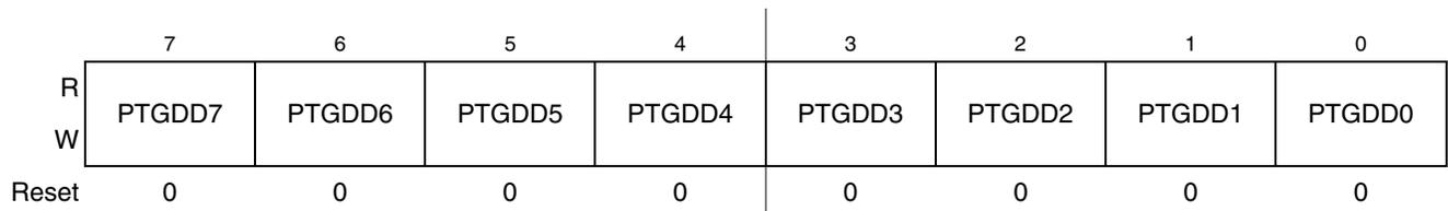
Figure 6-36. Data Direction for Port G (PTGDD)
