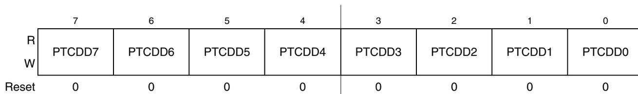
**Figure 6-20. Data Direction for Port C (PTCDD)**
