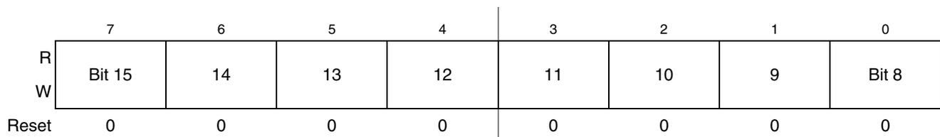
**Figure 10-11. Timer x Channel Value Register High (TPMxCnVH)**
