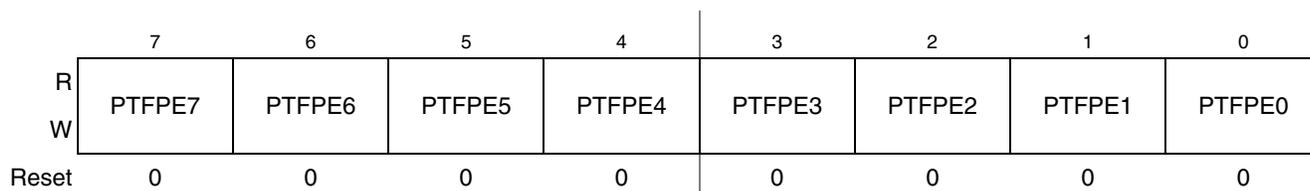
Figure 6-30. Pullup Enable for Port F (PTFPE)
