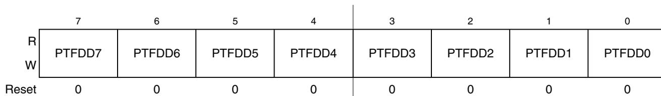
Figure 6-32. Data Direction for Port F (PTFDD)
