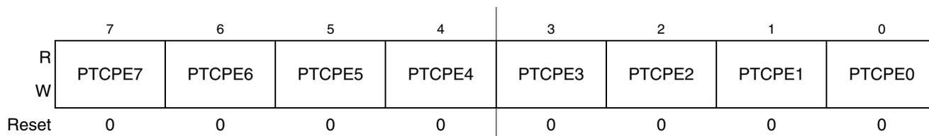
**Figure 6-18. Pullup Enable for Port C (PTCPE)**
