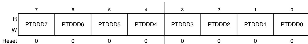
Figure 6-24. Data Direction for Port D (PTDDD)
