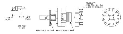
**NOTE:** Switches with 'C' or 'MC' terminations have additional terminal no. 9 as switch support only. This terminal is not connected electrically inside switch. Solder and clean switch base on PC board with other components, then snap on housing/actuator assembly. See page K-7 for installation instructions.
