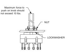
Install switch with stop ring (if used) and lockwasher in back of panel. Tighten hex nut from front of panel.
