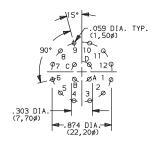
4P MODEL SP MODEL (omit terminals B, C & D) DP MODEL (omit terminals B & D)
