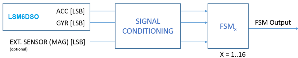
Figure 2. State machine in the LSM6DSO
