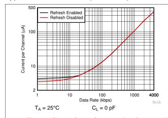
Figure 7. ISO7041 Supply Current vs Data Rate at 3.3 V (With No Load)
