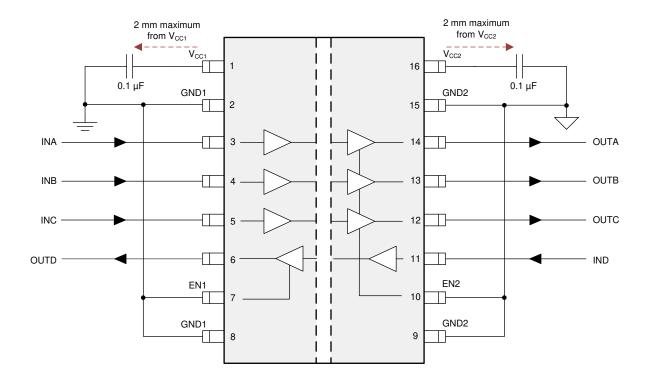
Figure 19. Typical ISO7041 Circuit Hook-up
