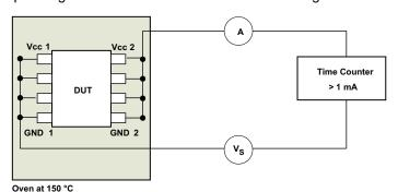
Figure 16. Test Setup for Insulation Lifetime Measurement
