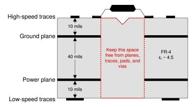
Figure 24. Recommended Layer Stack
