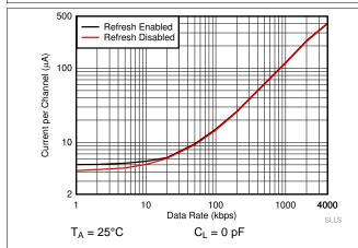
Figure 9. ISO7041 Supply Current vs Data Rate at 5 V (With No Load)
