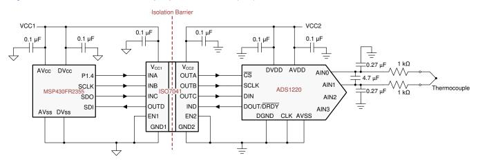
Figure 18. Isolated SPI for a Temperature Field Transmitter
