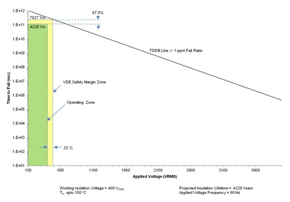
Figure 17. Insulation Lifetime Projection Data
